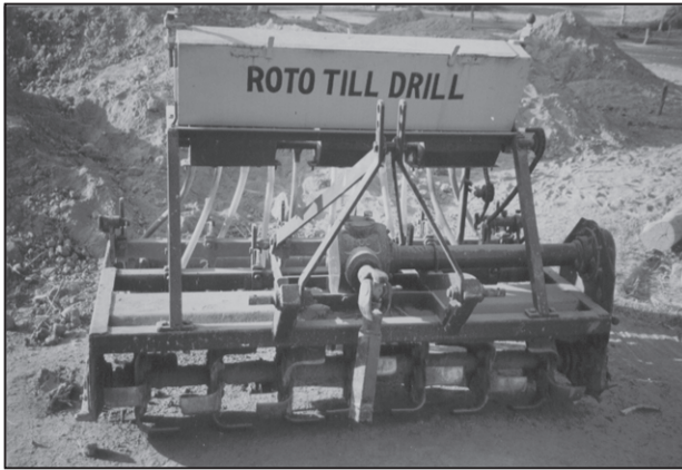
Fig. 5.12 : Roto Till Drill—A modern agricultural equipment
