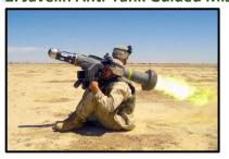
India and the US recently announced plans to pursue new procurements and co-production arrangements for Javelin anti-tank guided missiles, to meet the defense requirements of India. It is a man-portable, fire-and-forget, anti-tank guided missile. It has an effective range of 2.5 km. It is a fire-and-forget missile with lock-on before launch and automatic selfguidance. It uses automatic infrared guidance that allows the user to seek cover immediately after launch.
