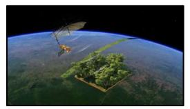
An European Space Agency mission to measure global forest biomass and understand the carbon cycle. Will generate 3D maps of dense and remote tropical forests. Launch via Vega C rocket from French Guiana into a sun-synchronous orbit at ~666 km altitude. First satellite to carry a P-band radar, enabling deep forest canopy scanning. Captures data on trunks, branches, and stems where most carbon is stored. Aims to assess forest height, above-ground biomass, and monitor forest changes from space.
