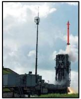
Medium Range-Surface to Air Missile (MR-SAM) is a high-response, quick-reaction, vertically launched supersonic missile for neutralizing aerial threats. Developed by Defence Research and Development Organisation (DRDO) and Israel Aerospace Industries; produced by Bharat Dynamics Limited (BDL). System includes command and control unit, tracking radar, mobile launcher, and missiles.
